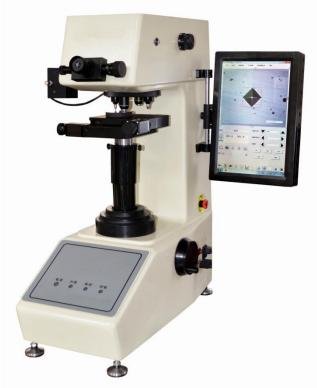
New generation of automatic Micro Vickers hardness tester adopts the integrated design of hardness tester and panel computer with Windows 7 operating system.
